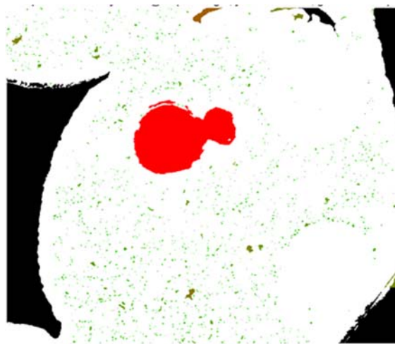
Fig. 6. Pore density map of a micrograph of the struts orthogonal to the cross-section.
