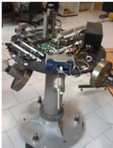
Fig. 1.b. Simulator with ACS components and spherical air bearing [21]
