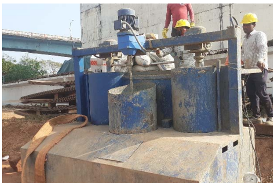
Fig. 2. Twin drum grouting mixer with additional agitator
