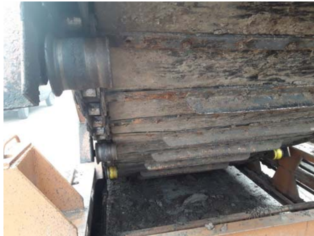
Fig. 5. Mounted support roller, Bottom: polyurethane sheath, Top: Gray cast iron GG 20
