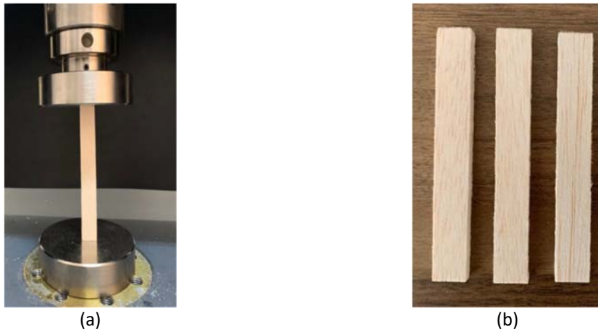
Fig. 4. a) Axial compression test setup. b) Axial compression test samples.
