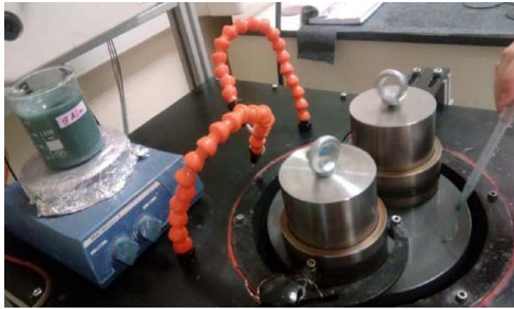
Fig. 1. The grinding process of specimens in the lapping machine.
