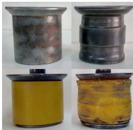
Fig. 6. Unworn and worn gray cast and polyurethane sheath support roller bearing hubs
