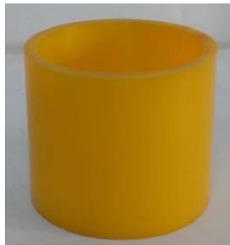
Fig. 4. Hot-cast polyurethane elastomer sheath
