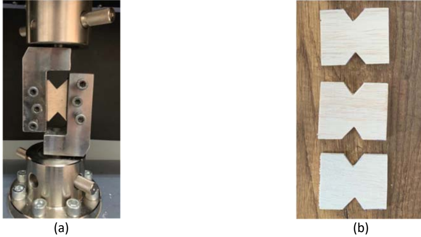
Fig. 3. a) Shear test setup. b) Shear test samples.
